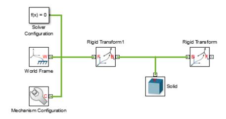
5 In the Solid block dialog box, specify the following parameters. Later, you define the MATLAB variables shown using a Subsystem block that contains the Solid and Rigid Transform blocks. Among its advantages, this approach enables you to update variables used in multiple blocks from a single place—the Subsystem block dialog box.
