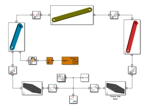
To specify the force or torque acting at a joint, Simscape Multibody provides a selection of actuation inputs directly in the joint blocks. Each joint primitive—the basic component of a joint block—provides a selection of actuation inputs specific to that primitive.
